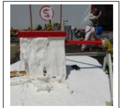
" Wind protected" Foam pourer test
